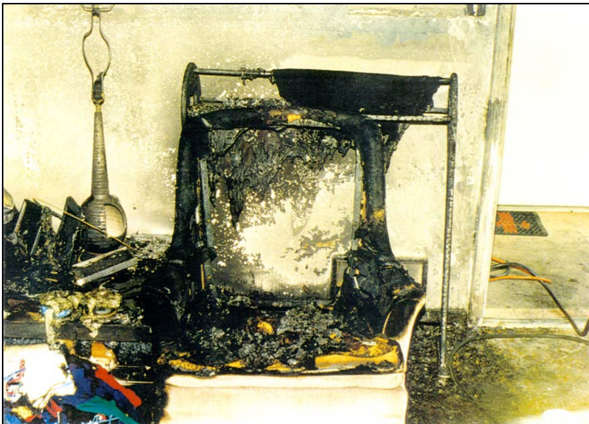
Figure 28: Table Lamp Undisturbed after Fire Self Extinguished
