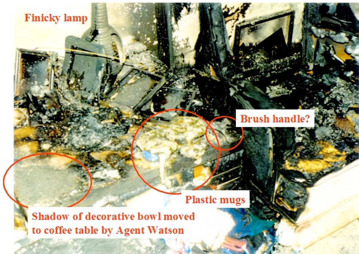
Figure 67: No Evidence of Candles or Candle Holders on End Table
