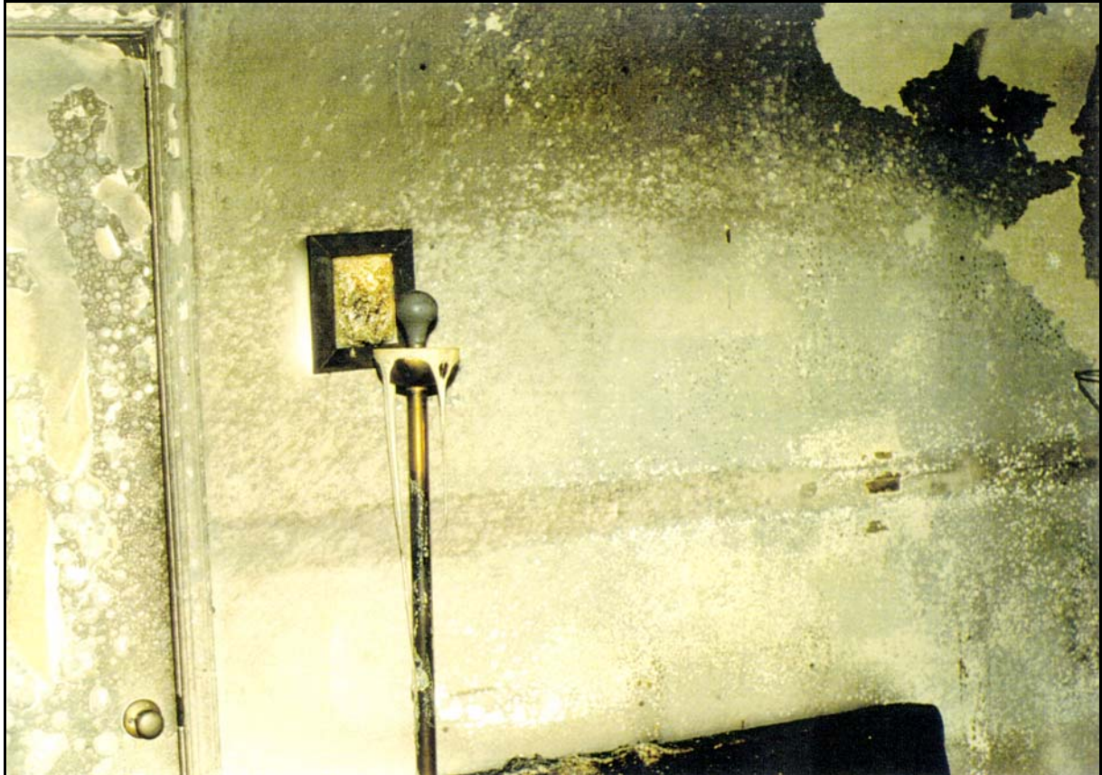
Figure 29: Light Bulb in Floor Lamp Undamaged by Light Bulb
