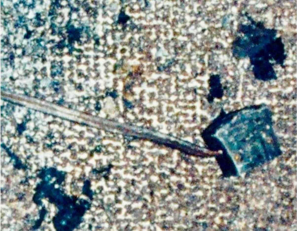
Figure 54: Lamp Cord Plug with Prongs Missing
