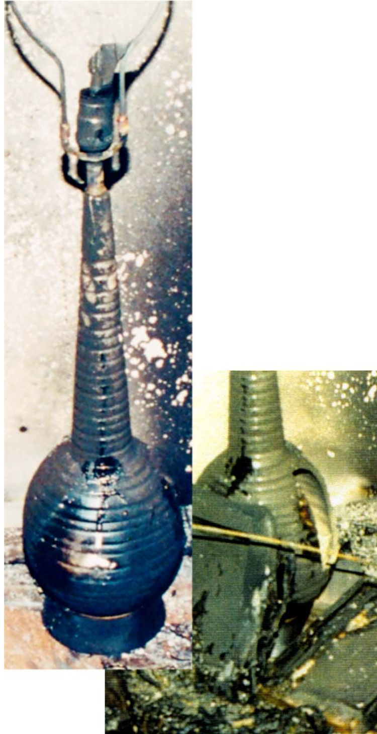
Figure 30: Melt Stains Running Down Side of Table Lamp
