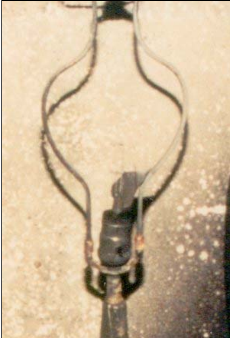
Figure 27: Close up of Table Lamb After Fire -- Light Bulb Exploded
