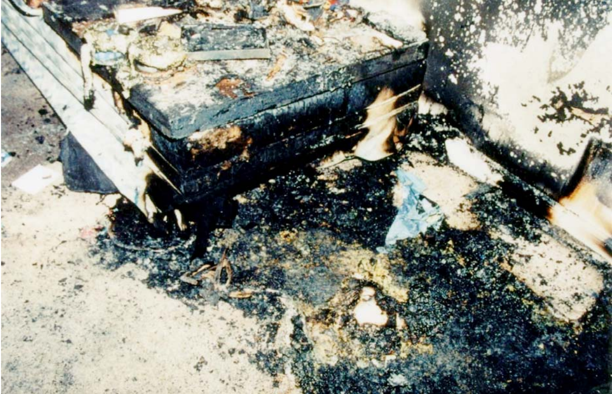
Figure 24: Insurance Investigator's Photo of Presumed Fire Origin -- Carpet Sample Not Yet Removed
